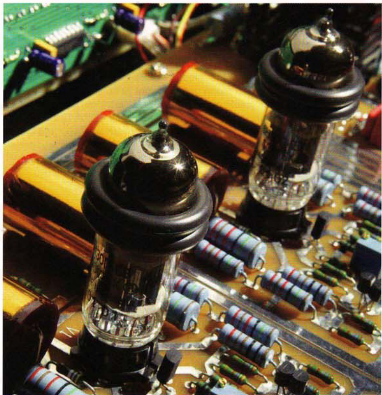
ABOVE: Damping rings are used to control microphony in the 6H30 double-triodes
